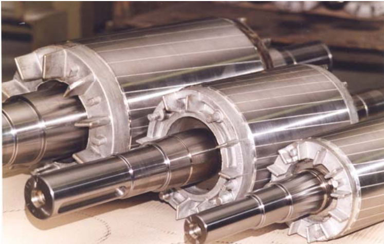
Pict. 3: Rotors of norm motors with aluminium die-cast squirrel cage
