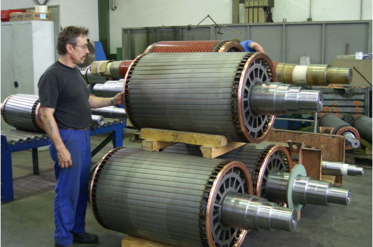
Pict. 6: Rotors of transnorm motors with copper-bar cage
